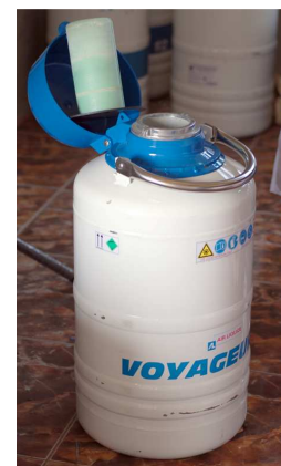
Figure 19: Liquid nitrogen tank suitable for field use (Photo: Herbreteau V.)
