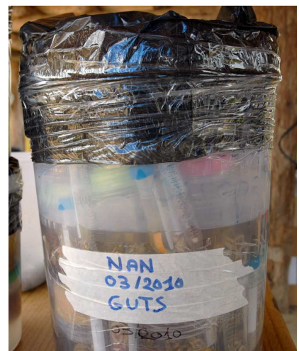
Figure 65: Preservation of Falcon tubes in a container filled with 70% ethanol to avoid evaporation (Photo: Herbreteau V.)
