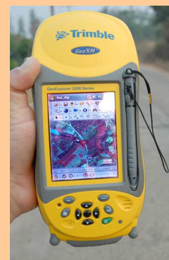
Figure 5: GPS receiver with integrated GIS software (Photo: Herbreteau V.)
